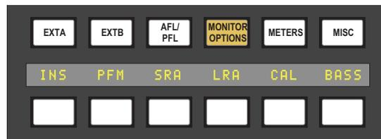
**INS** – This switches the encoder/decoder insert into the monitor path for use with 5.1 monitor sources selected via the EXT A monitor selector.
