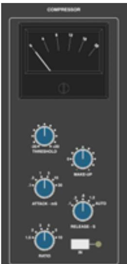
Selecting the **IN** button to switch the compressor into circuit introduces no additional audio circuitry to the main outputs.
