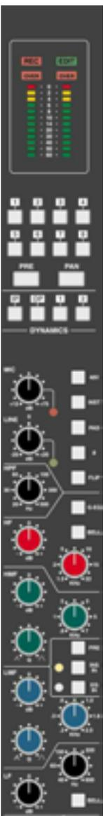
Three buttons – IP, OP, **1** and PRE **2** are used to determine where each processor will be placed in the signal chain. Three additional buttons are provided to switch each device into circuit:
