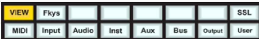
**Fkys** are the eight functions keys as on the HUI interface. These are also permanently mapped to the numeric keypad, which is not supported in the Mackie Control protocol.
