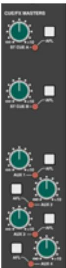
An **AFL** button is provided for each output. The AFL signal is intelligently assigned to left and right AFL busses. Selecting AFL on a single FX output will route signal to both left and right AFL busses. Selecting AFL on odd and even numbered FX outputs will route the odd numbered output to the left AFL bus and the even numbered output to the right AFL bus.
