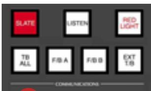
**5 RED LIGHT** – this provides an isolated contact closure for hooking up to a studio red light via an external relay box. This function can be fired from a GPI input (see Section 3 for details).
