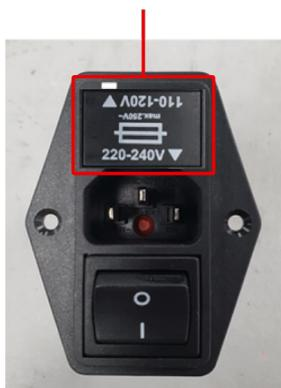
*The fuse cartridge holder on some Fusion units may differ to what's described above. Always check the fuse information on the rear of your physical unit to verify you are inserting the correct fuses when changing the operational voltage.*
