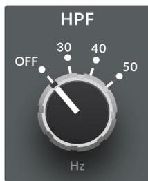
The High-Pass Filter allows you to reduce sub frequency content in your mix. The filter is a 3rd order/18dB per octave slope. The pot is stepped and allows you to choose between four fixed settings - OFF, 30Hz, 40Hz and 50Hz. OFF or 30Hz are often suited to whole mix material, whilst the 40Hz and 50Hz can help remove unnecessary rumble when processing individual instrument stems. Removing this low-energy from stems can give you back some headroom in the overall mix.
