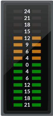
A master meter, with three second peak hold allows you view the main output level of Fusion. The scale is referenced in dBu, with +24dBu at the top. The aim of the game is not to max out this meter - typically full mix material would be peaking between +9dBu and +15dBu, occasionally as high as +18dBu. Ensure that the output level of Fusion does not exceed the operating input level of your A/D converter, otherwise it will clip.
