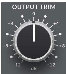
The **OUTPUT TRIM** provides  $\pm 12$ dB gain at the output stage of Fusion. This pot is indented at the 12 o'clock position. This control is important in order to compensate for any level increases caused by the preceding sections.
