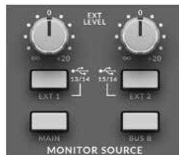
The EXT inputs show a USB symbol, this is because the EXT inputs can be sourced from the USB D/A returns. A pair of switches next to the TALK LEVEL knob allow the EXT 1 and EXT 2 signals to be sourced from USB Returns 13/14 and 15/16 respectively. These switches over-ride the External Input TRS Jacks.
