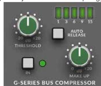
The bus compressor side chain also has a 1st order High Pass Filter at approx 50 Hz, a feature of more modern SSL bus compressor designs to give smoother performance from mixes with prominent bass content.
